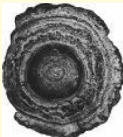
Fe-Mn oxide layers around the nucleus of the nodule
